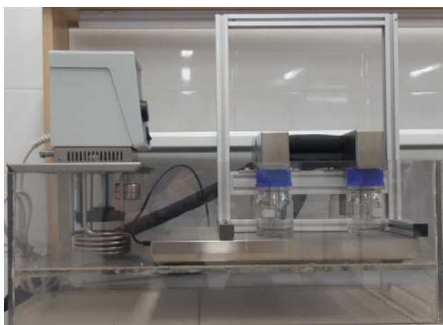
Figure 3. The Cold Finger laboratory unit CF-4
