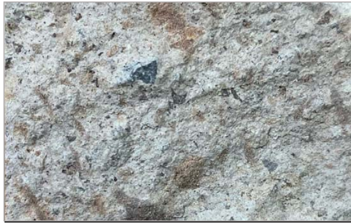
Figure 3. Overburden volcanic tuff structure
