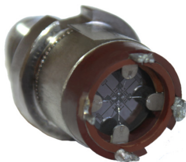
Figure 1. Semiconductor strain gage on the structure of CSN
